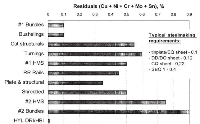
Figure 2—Typical residual content of scrap. (Source: Scarnati<sup>13</sup>)
