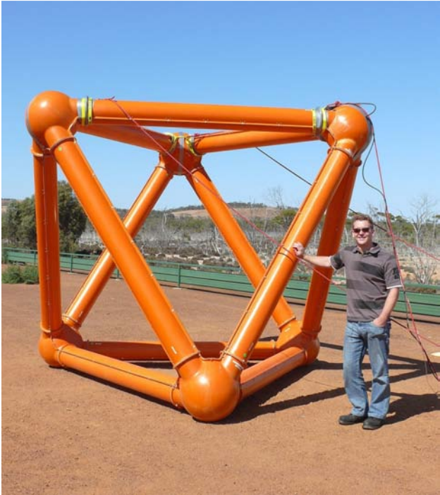
Figure 3 Russell Mortimer from Southern Geoscience and the ZTEM base station
