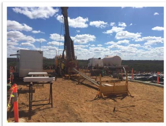
Figure 1 Photo of diamond drill rig at QVR preparing to start drilling QVD15
